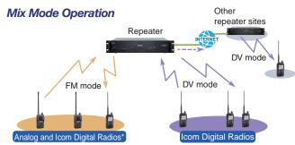
\* Icom digital radio can receive both FM and DV mode signals.
