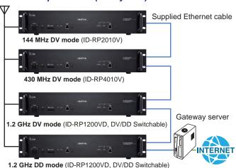
Up to 4 modules can be connected to one gateway server.
