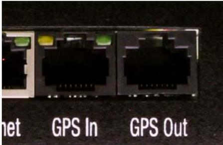
The RackInjector is able to receive a synchronization signal from a PacketFlux GPS receiver (SyncBox or SyncPipe). If you are intending to utilize one of these devices with the RackInjector, it can be connected at this point. Simply use a straight through CAT5 cable from the GPS receiver to the GPS In port.
