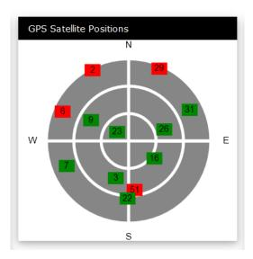
**GPS Satellite Positions:** This section of the screen is used to determine if you are having visibility problems with a portion of the sky.
