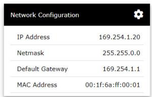
**Network Configuration.** This section allows you to display and set the network addresses for the RackInjector. It contains the following information:
