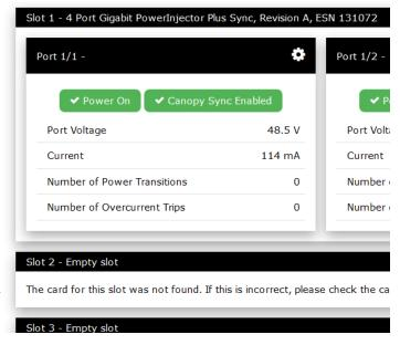
If a slot contains a board, the type of board and the board's serial number is displayed. Each port controlled by that slot is also displayed.
