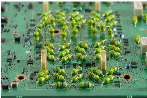
Figure 04-17. BPF circuit in the RF-B unit
