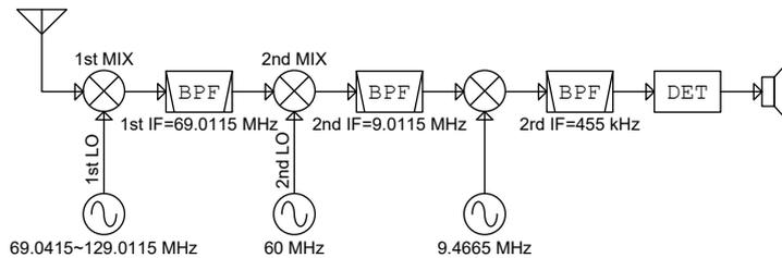
**Figure 02-5.** Receiver configurations of previous analog type radios
