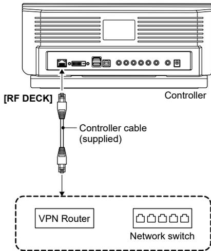
Figure 09-31. Connection with network switch or VPN router (2)
