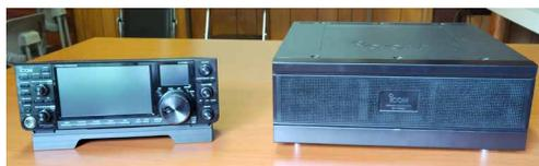
The Controller with the stand and the RF Deck.
