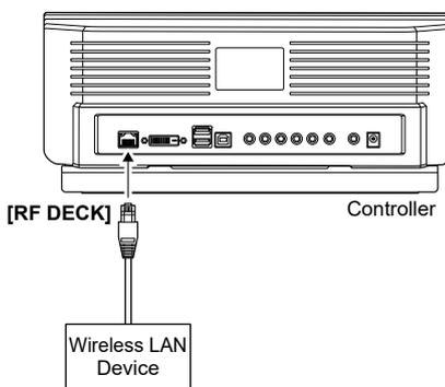
Figure 09-12. Connecting the Wireless LAN Device
