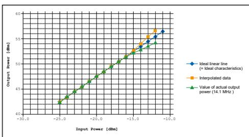
Figure 03-2. Linearity characteristics of the power amplifier
