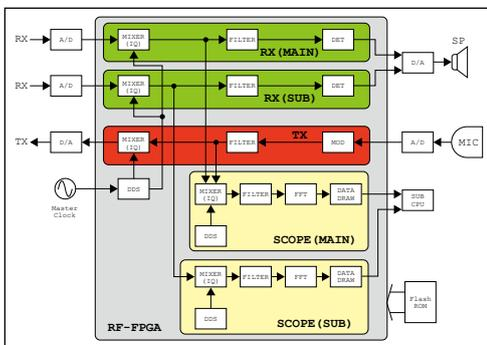
Figure 04-2. Block diagram of inside the FPGA
