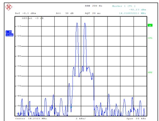
**Figure 05-27.** Transmit IMD characteristics when DPD is activated
