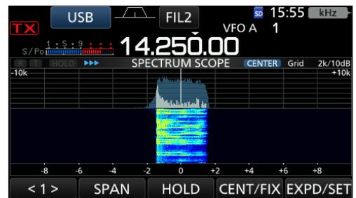
**Figure 05-5.** Receive signal spectrum when DPD is ON
