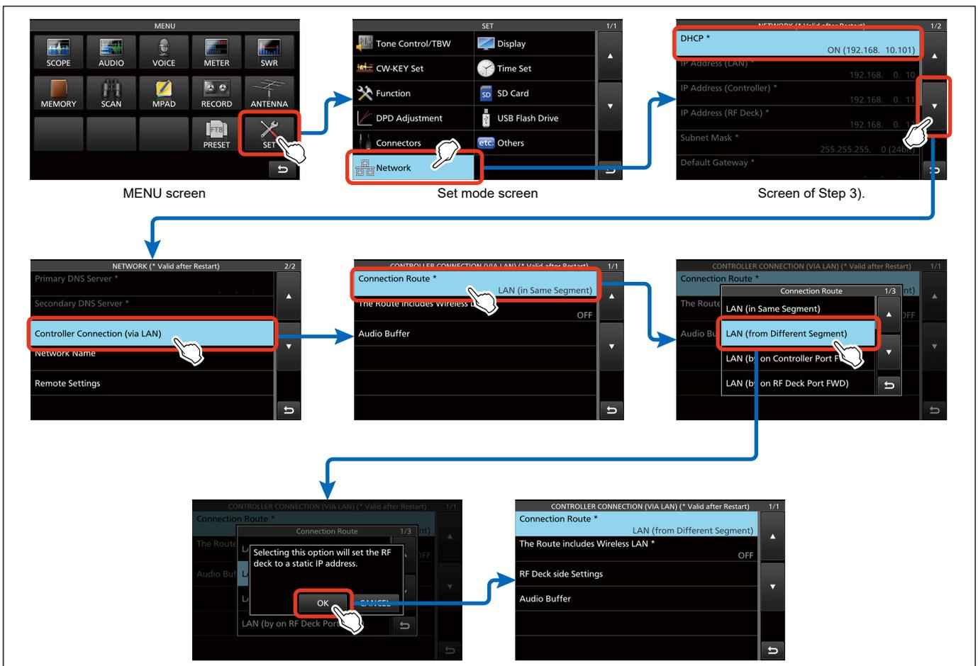
Figure 09-35. Flow of confirmation and setting— Home LAN (separate segment) connections (1)
