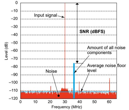
Figure 04-21. Basic idea of Signal-to-Noise Ratio (S/N).
