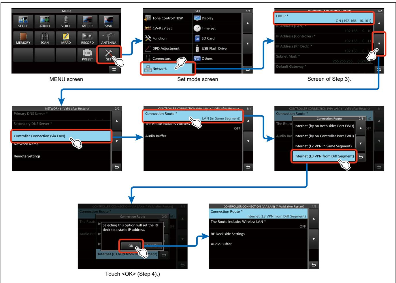
**Figure 09-24.** Flow of confirmation and setting— L3 VPN connections (1)
