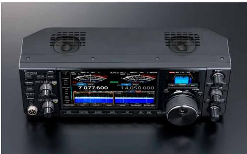
**Figure 04-26.** Main and Sub speakers are located on the top panel
