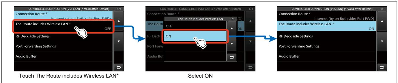
Figure 09-21. Configuration flow regarding wireless LAN
