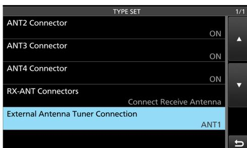
Figure 05-19. Screen of the antenna Set mode
