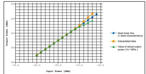
**Figure 05-24.** Input/Output characteristics of the IC-7760 RF power amplifier
