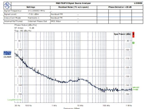
Figure 05-38. Transmit phase noise characteristics on the 14 MHz band
