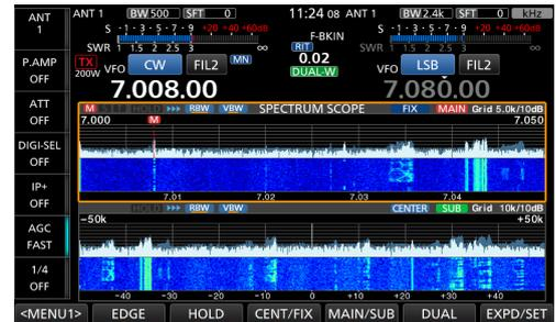
Figure 06-15. The Dual Spectrum Scope
