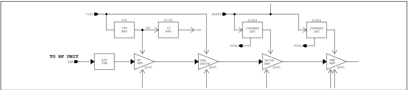
Figure 05-9. Block diagram of the PA unit
