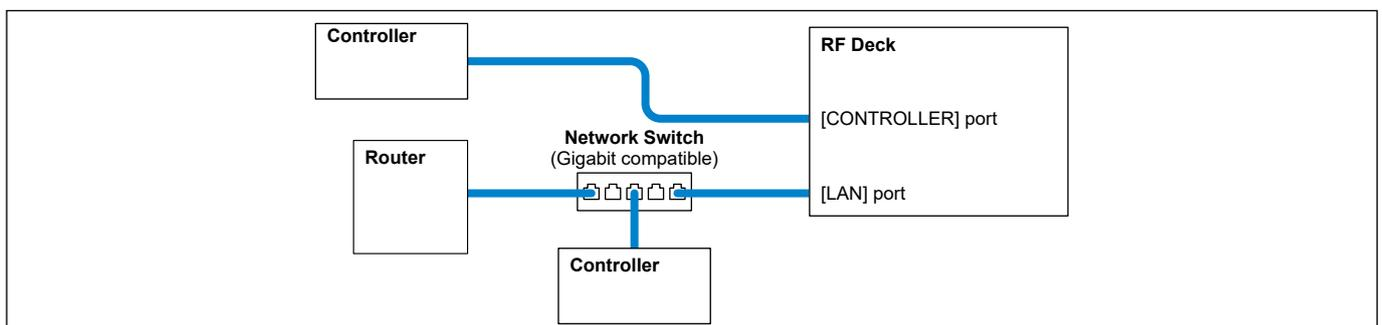
**Figure 08-3.** Direct connection and a connection through a LAN
