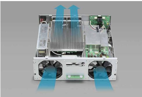
**Figure 05-14.** Cooling air flow
