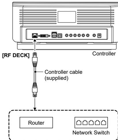
**Figure 09-43.** Connection to the network switch
