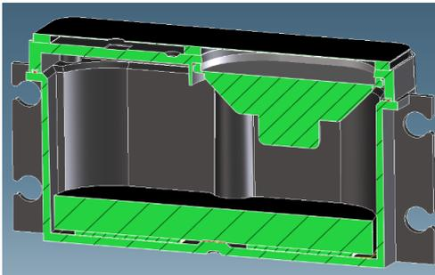
**Figure 04-27.** Cross-sectional view of the speaker box
