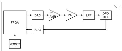
**Figure 05-25.** Block diagram of the DPD control circuit
