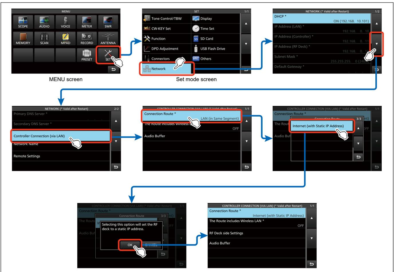
Figure 09-41. Flow of confirmation and setting— Internet connection (specifying static IP address) (1)
