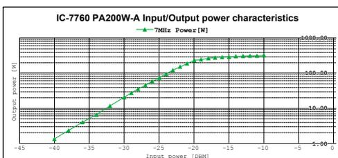
**Figure 05-12.** PA input/output characteristics of the IC-7760
