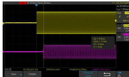
IC-7610: Approximately 9 msec. delay under the same test conditions to the left
