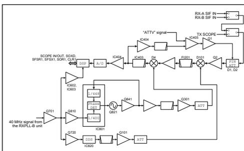
Figure 06-18. Block diagram of the IC-7700/IC-7800 Spectrum Scope
