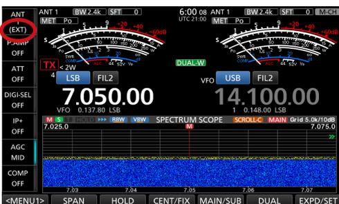
Figure 05-18. "EXT" displays when the AH-730 is connected
