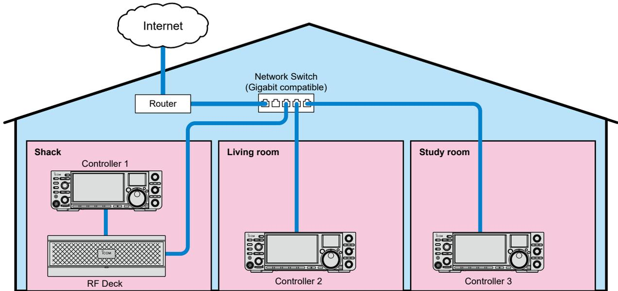
Figure 08-4. Connections with multiple Controllers through a switch (1)
