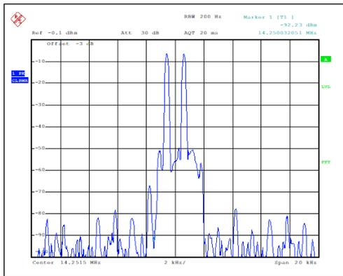
**Figure 05-3.** Transmit IMD characteristics with DPD ON
