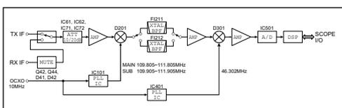
Figure 06-19. Block diagram of the IC-7850/7851 Spectrum Scope
