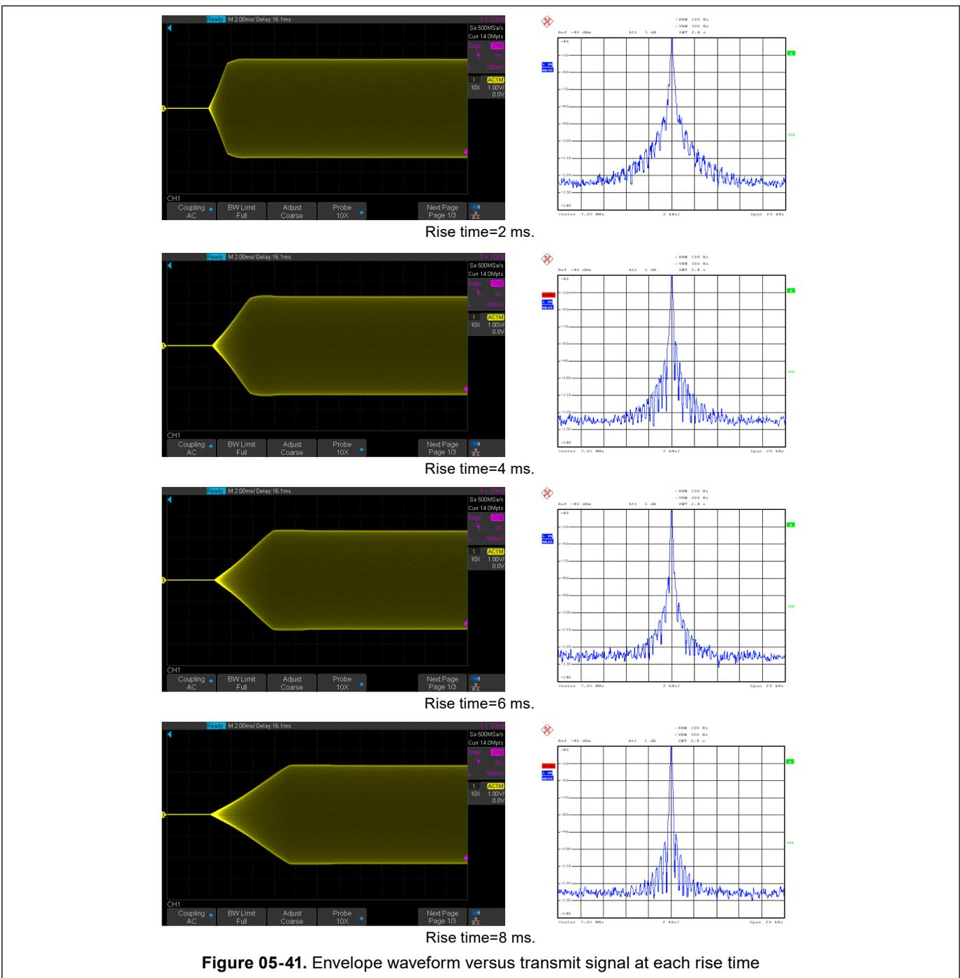
Figure 05-41. Envelope waveform versus transmit signal at each rise time
