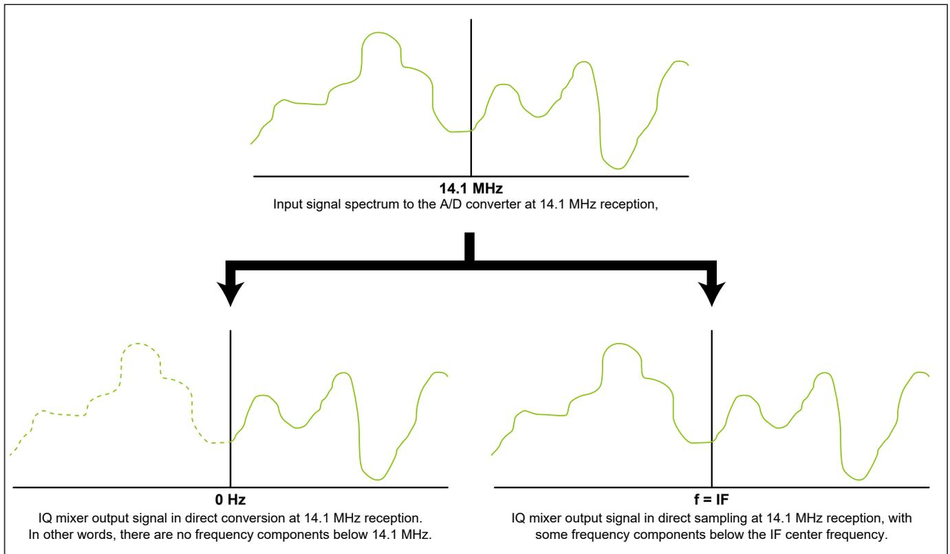
**Figure 04-4.** Difference between direct conversion and direct sampling
