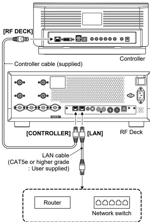
**Figure 09-13.** Connection with network switch or router (1)
