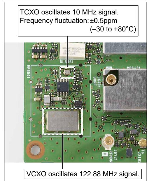
Figure 06-8. TCXO and VCXO installed in the IC-7760
