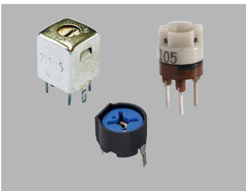
Figure 02-4. Analog components for adjustments
