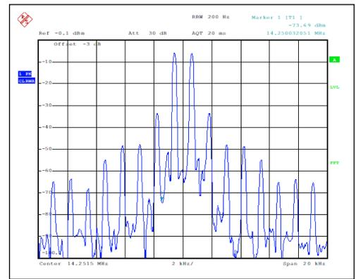
**Figure 05-2.** IC-7760 transmit IMD characteristics with DPD OFF
