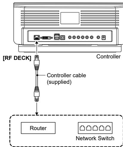
**Figure 09-17.** Connection with network switch or router (2)
