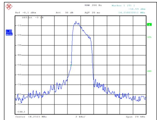
**Figure 05-29.** IC-7760 pseudo voice spectrum/DPD is activated (ON)
