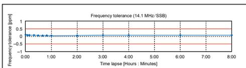
Figure 05-7. Frequency tolerance on SSB at 14.1 MHz
