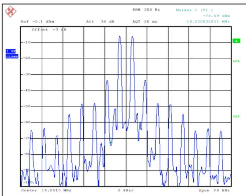
**Figure 05-26.** Transmit IMD characteristics when DPD is OFF
