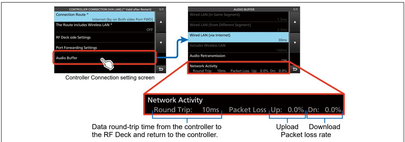
**Figure 09-49.** Checking the Network Activity
