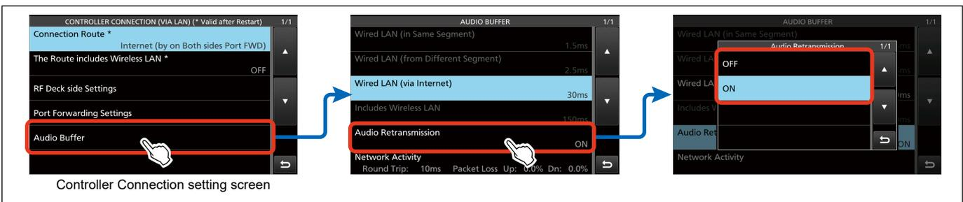
Figure 09-48. Audio Retransmission function setting flow
