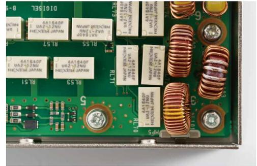
**Figure 04-14.** High Q coils used in DIGI-SEL with toroidal cores
