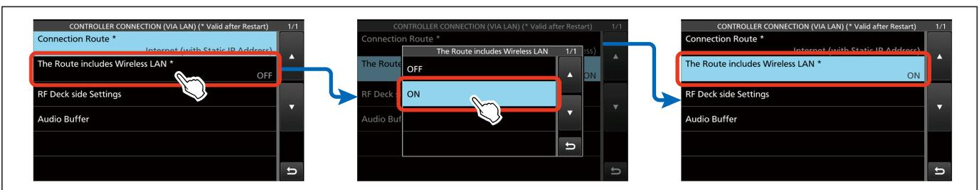
**Figure 09-46.** Flow of confirmation and setting— Internet connection (specifying static IP address) (4)
