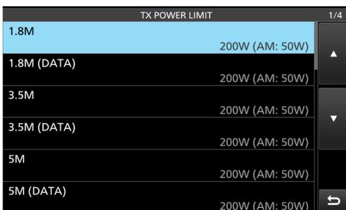
**Figure 07-15.** Transmit output power limit setting screen
