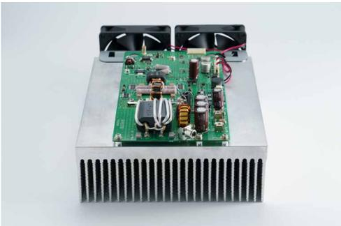
Figure 05-10. PA unit of the IC-7760
