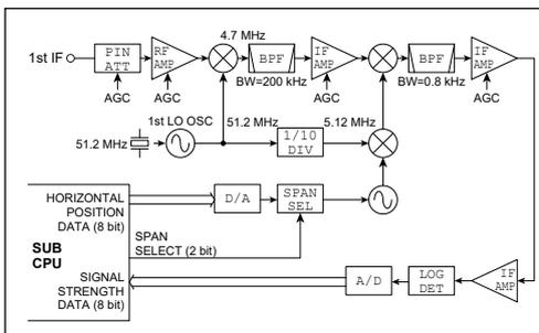
Figure 06-17. Block diagram of the IC-780 Spectrum Scope
