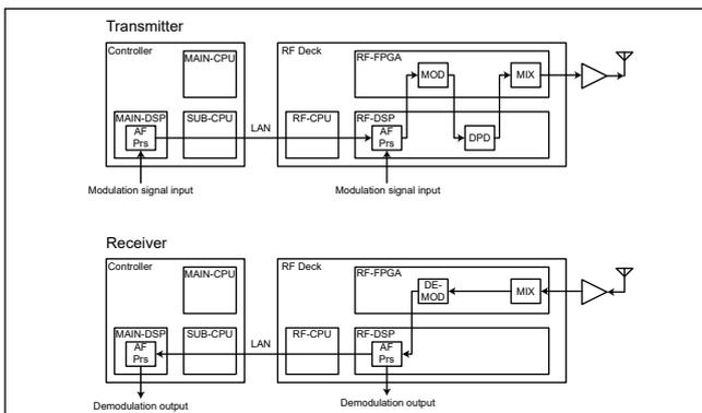
**Figure 04-24.** Block diagram of FPGA and DSP
