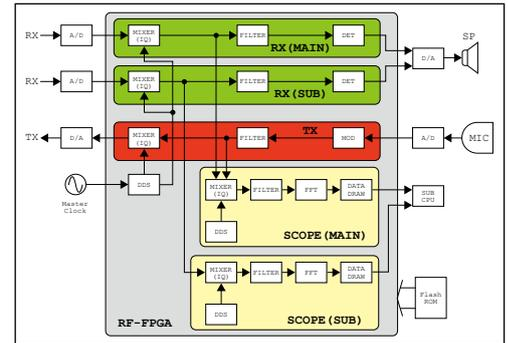
Figure 04-8. Block diagram of inside the FPGA
