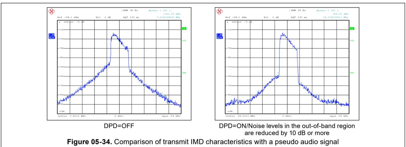
**Figure 05-34.** Comparison of transmit IMD characteristics with a pseudo audio signal
