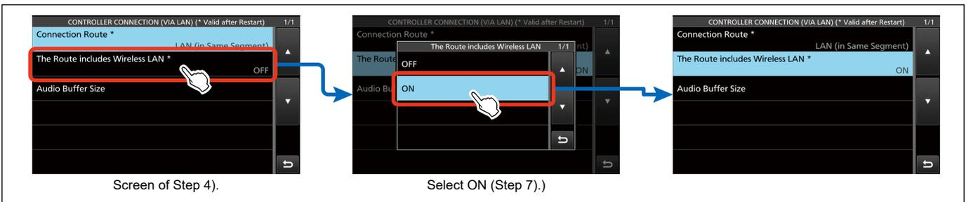
Figure 09-11. Configuration flow for wireless LAN
