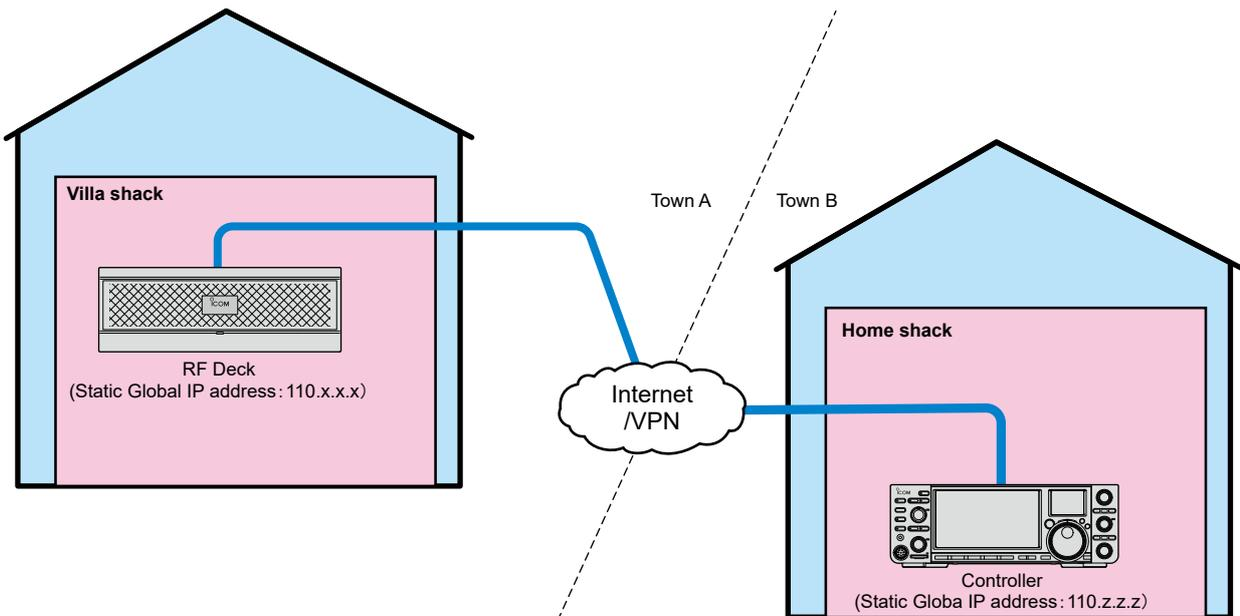
Figure 09-6. Internet connection with a static IP address
