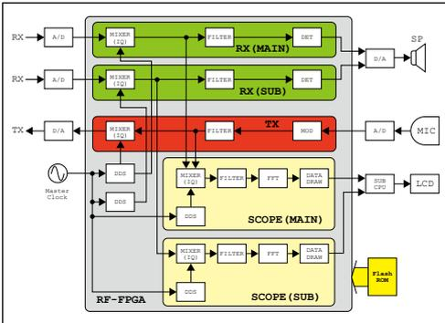
**Figure 06-20.** Scope block diagram for the IC-7760
