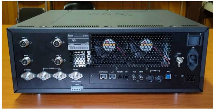
Figure 07-2. Rear panel of the RF Deck
