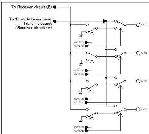
Figure 06-4. Block diagram of the antenna switching circuit
