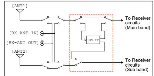
**Figure 04-10.** Block diagram of the splitter circuit
