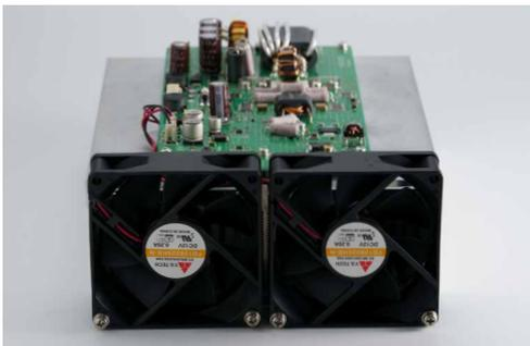
**Figure 05-15.** Two large cooling fans are installed on the PA unit
