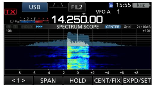
**Figure 05-4.** Receive signal spectrum when DPD is OFF
