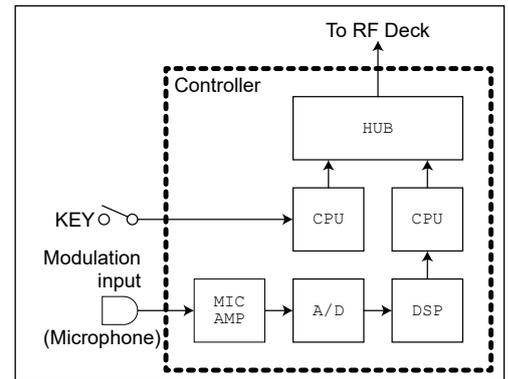
Figure 05-42. Block diagram of the internal Controller unit
