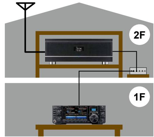
Figure 03-3. Example connection through a network switch
