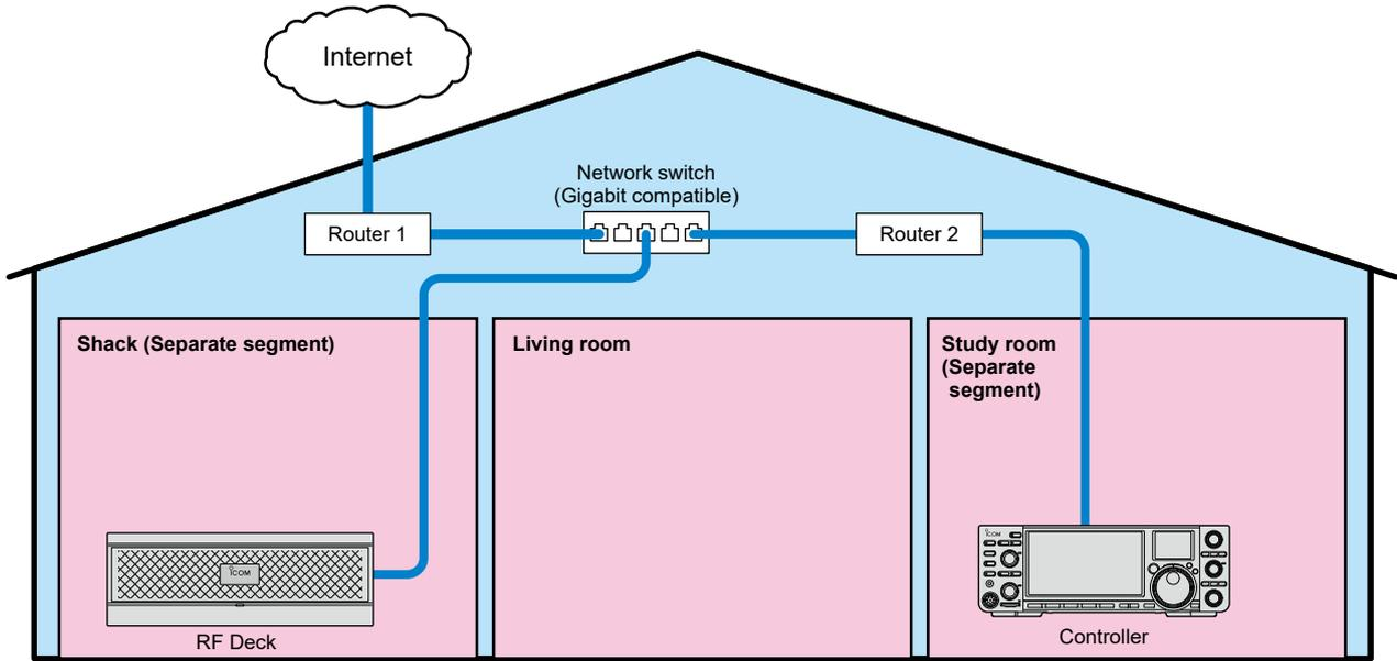
Figure 09-5. Home LAN (home network) connection with separate segment settings
