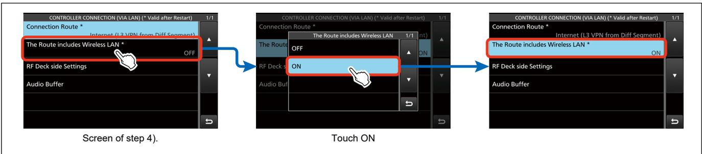
Figure 09-27. Configuration flow regarding wireless LAN
