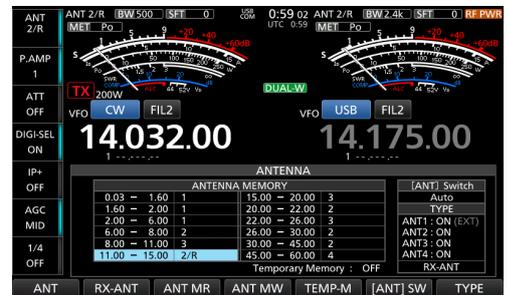
Figure 06-5. Antenna settings per band
