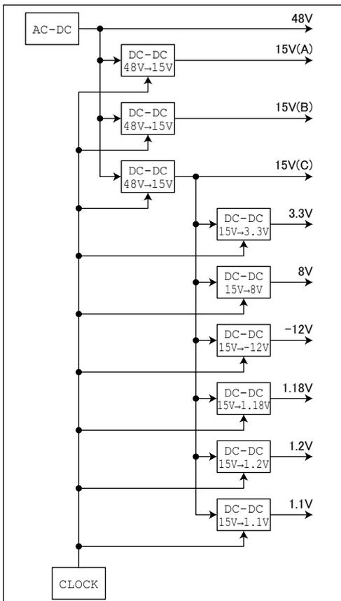
Figure 06-2. Block diagram of the Power supply unit
