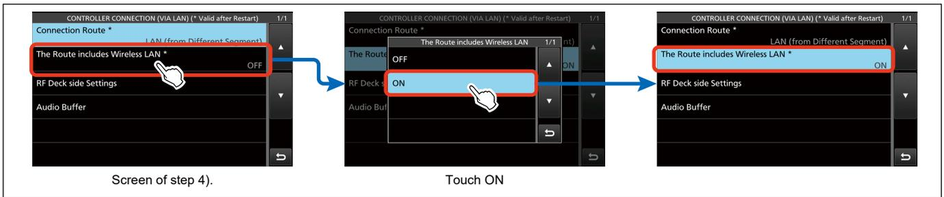
Figure 09-38. Configuration flow regarding wireless LAN
