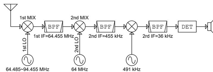
**Figure 02-6.** Receiver configuration of the early DSP radios
