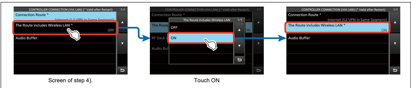
Figure 09-32. Configuration flow regarding wireless LAN
