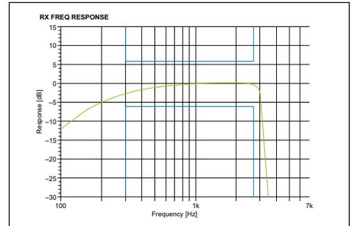
**Figure 04-3.** Characteristics of HPF for audio frequency
