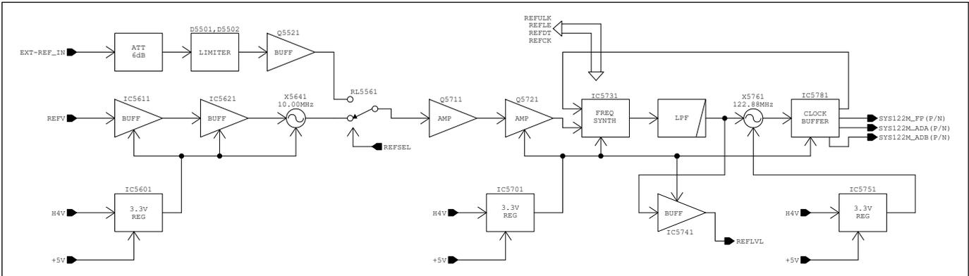
Figure 06-7. Block diagram of the sampling clock generator
