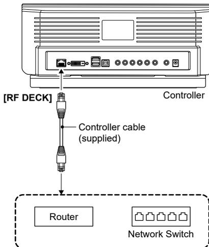
**Figure 09-37.** Connection with network switch or router (2)
