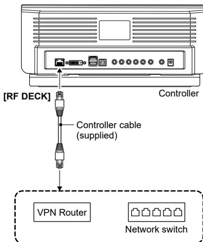
**Figure 09-26.** Connection with network switch or VPN router (2)
