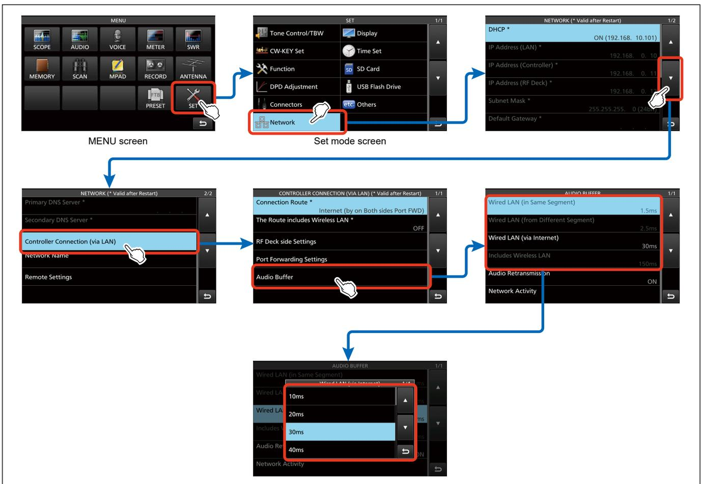
Figure 09-47. Flow of setting the audio buffer
