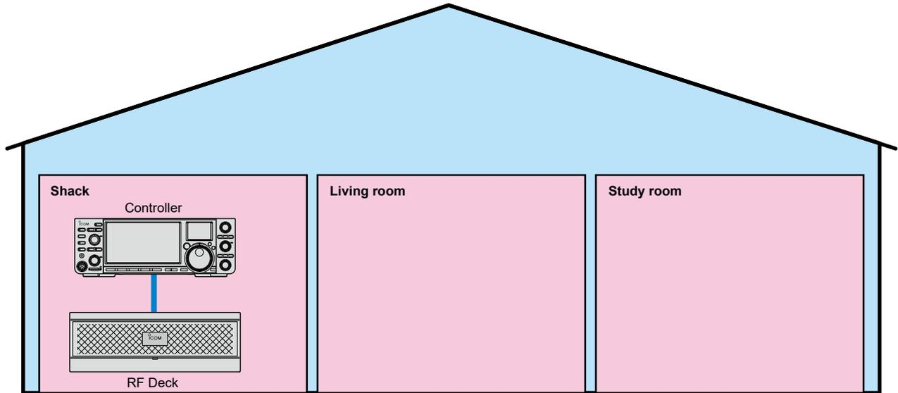
Figure 09-1. Direct connection
