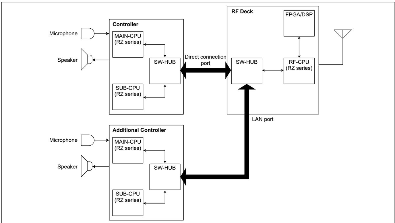
**Figure 08-1.** Network block between Controller and RF Deck
