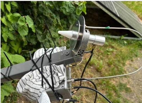
Figure 07-17. POTY feed and CX-10G attached to the offset dish
