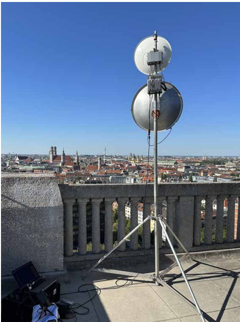
Figure 07-15. High above the rooftops of Munich: The 10 GHz transverter CX 10G (top) the RF unit with dish antennas for 3 cm (10 GHz) and 13 cm (2.4 GHz) on the mast. The control unit is offset from this.
