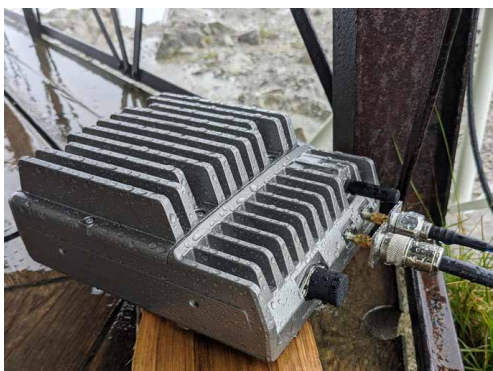
Figure 07-11. The RF unit - waterproof
