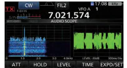
FFT scope + Oscilloscope
