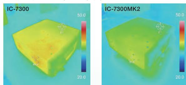
\* Device left in RX standby mode for 6 hours at 24°C room temperature.
