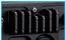
The rear panel is covered with thermosetting resin coating to resist corrosion.
