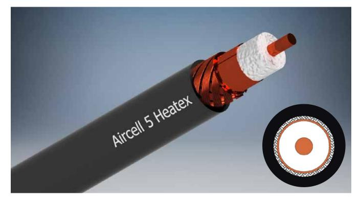
Aircell 5 Heatex is a flexible and thin coaxial cable with 5 mm outer diameter for the frequency range from DC to 10 GHz. Its low loss characteristics and the ability to use standard RG 58 connectors make this cable the number one choice not only for Wireless LAN applications but also for general RF communications.
