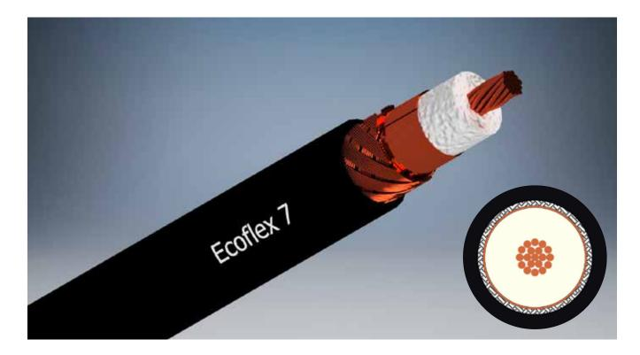
Ecoflex 7 is an ultraflexible coaxial cable designed for frequencies up to 6 GHz. Due to its extraordinary low loss in relation to the outer diameter and the small bending radius the cable can be used for numerous RF applications.
