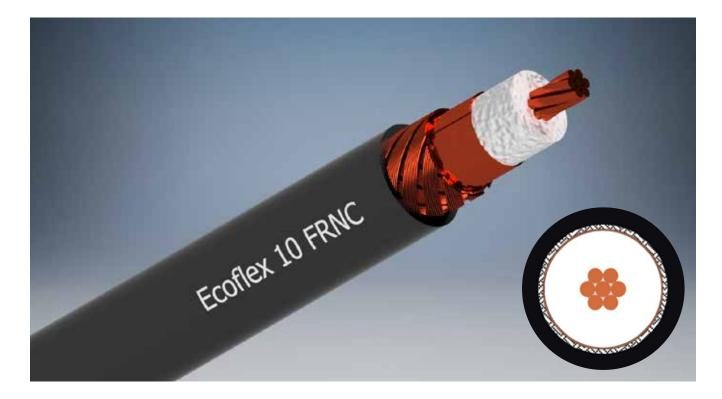
Ecoflex 10 FRNC is a flexible, low loss 50 ohm coaxial cable for the frequency range up to 6 GHz. Advanced manufacturing techniques combined with the use of a low loss PE-LLC dielectric with a foaming rate of more than 70% result in very low attenuation values, which set standards among flexible coaxial cables of this dimension.
